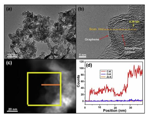
Fig. 4. (a) TEM images of the tribofilm debris. The graphene layered nanoscroll structures were observed on HRTEM bright field images (b) and dark field images (c), insert is the line scan range (the scanning direction is from left to right). (d) Line scanning of C, O, Al atoms. (A colour version of this figure can be viewed online.)
