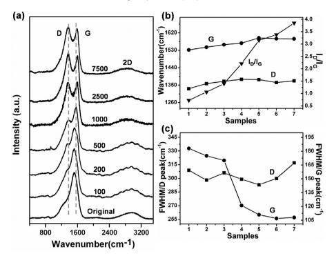
Fig. 3. (a) Raman spectra of tribofilms at different cycles, respectively. (b) G and D band position measured at 532 nm, and  $I_D/I_G$  of tribofilms at 0–7500 friction cycles. (c) The FWHM of D and G band.
