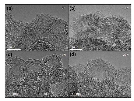
Fig. 6. HRTEM images of the tribofilm debris from Al<sub>2</sub>O<sub>3</sub> under different load at 2N, 5N, 10N and 20N, respectively.
