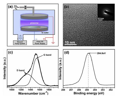
Fig. 1. (a) Model of the plasma-enhanced chemical vapor deposition (PECVD) technique. (b) High resolution transmission electron micrographs and electron diffraction pattern, and the selected area electron diffraction (SEAD) image. (c) Raman spectra and corresponding Gauss decomposition. (d) XPS C<sub>1s</sub> spectra of a-C: films spectra. (A colour version of this figure can be viewed online.)
