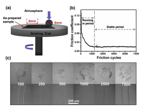
**Fig. 2.** (a) The schematic diagram of friction test machine with ball-on disk rotating mode. (b) Frictional curve of carbon films in the air with 20% humidity: the friction coefficient as a function of friction cycles. (c) The micrographs of  $Al_2O_3$  balls (top images) and a-C surfaces (bottom images) at 100, 200, 500, 1000, 2500, 7500 friction cycles, respectively. (A colour version of this figure can be viewed online.)
