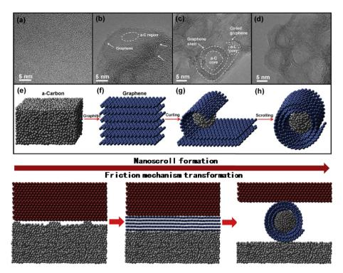
Fig. 8. (a) HRTEM images of original films. (b), (c) and (d) tribofilm debris of 200, 1000 and 7500 friction cycles, at 10N, 10 Hz. (e), (f), (g), (h), Schematic diagram of nucleation and growth model for GNSs. The bottom sketch map show the transformation of friction mechanism of friction interface. (A colour version of this figure can be viewed online.)
