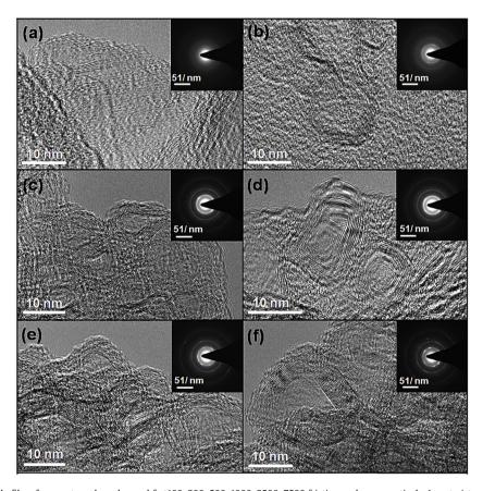
Fig. 7. HRTEM images of the tribofilms fragments: a, b, c, d, e and f at100, 200, 500, 1000, 2500, 7500 friction cycles, respectively. Insert pictures are the selected area electron diffraction of corresponding debris. Bottom table shows the corresponding friction coefficient at different friction cycles.
