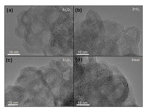
Fig. 5. HRTEM images of the tribofilm debris under different duality at 10N, 10 Hz.
